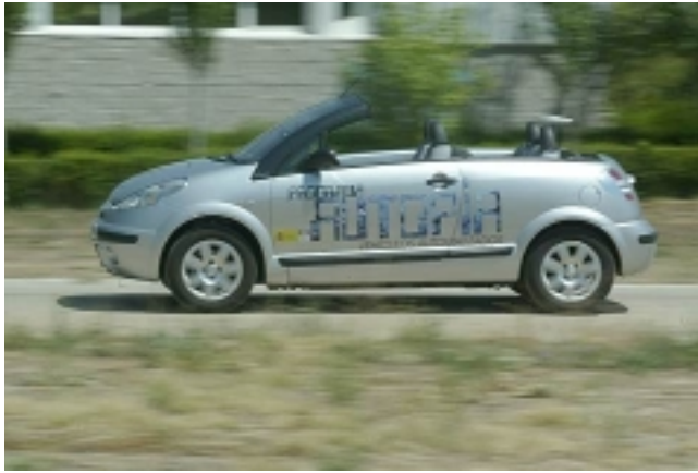
Fig. 1. Image of Clavilenyo automated vehicle in an autonomous trajectory. This is a Citroën C3 Pluriel whose actuators has been automated and equips an onboard computer and some sensors.
