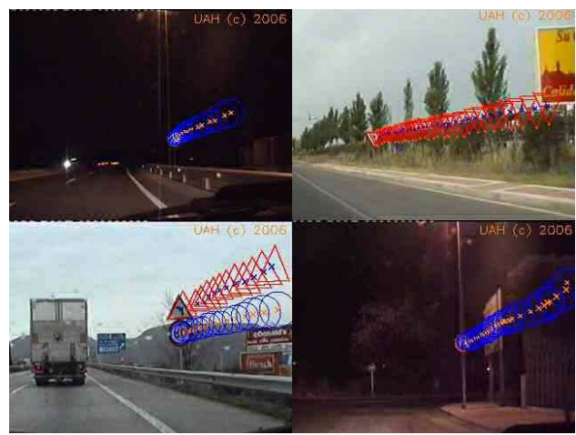
Fig. 4. Traffic-sign tracking under different lighting conditions using the Kalman filter. From left to right and up to down: end of forbidden overtaking at night. Give-way sign in a cloudy day. Left bend warning and speed limit sign in a cloudy day with rain drops on the car windscreen. Stop sign at night in the city.
