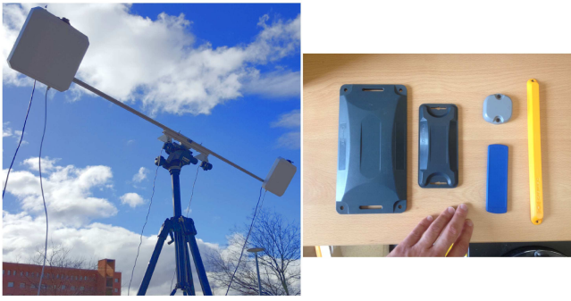
Fig. 4. Left: sensor setup, including two CMOS USB cameras and two far field circularly polarized panel antennas within the 865-870MHz band (Europe frequency allocation) located at the same baseline. Right: different passive RFID tags used in our experiments.
