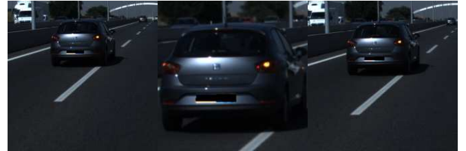
Fig. 5: Different ROI generation methods. From left to right: image size based, detection size based, and double detection size based.
